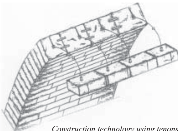
Construction technology using tenons and dowels sealed with lead Photo: Gilles Pequeux
